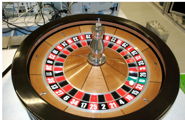
Fig. 1. The European roulette wheel. The standard roulette wheel consists of 37 pockets (numbered from 0 to 36) on a heavy circular disk mounted on a central pivot (the central portion of the wheel). This rotates with low friction on a fixed metal frame (the stator ) upon which are mounted several metal deflectors (on this model there are eight, one per eighth-sector of the wheel, mounted in the light wood panel rim). The sharp frets dividing the pockets on the rotating portion of the wheel introduce strong nonlinearity as the ball slows and bounces between pockets. The ball is shown in this figure at rest in pocket 32.
