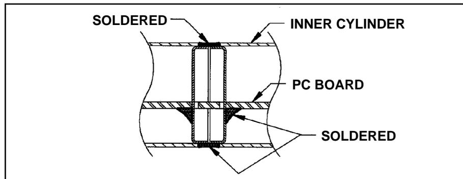
The soldered ground path technique provides much more stability to a trap notch over the life of the trap, than the separate cylinder design, held together through a mechanical fit.
